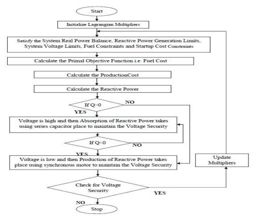
Fig. 1. Flowchart for Lagrangian Decomposition Approach
