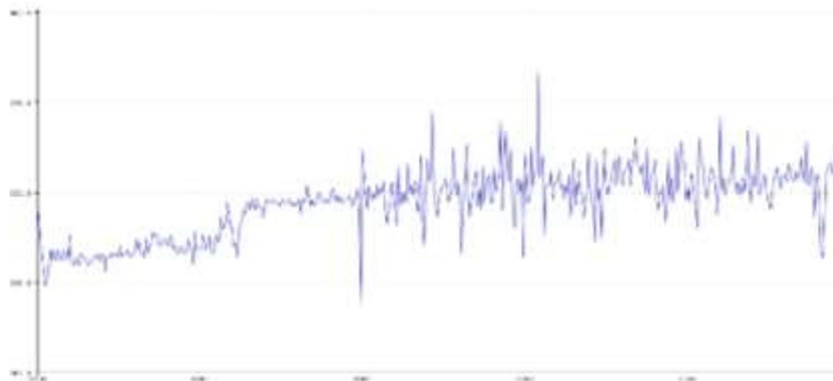
Figure 4: Temperature readings from a home automation system's DHT11 sensor are shown graphically.
