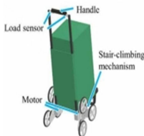
Fig 1. Carrying luggage in a Triple star wheel system
