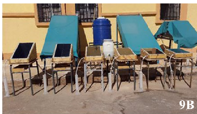
Fig.7B.Solar stills with different angles [9]
