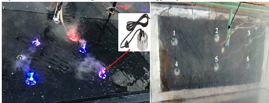
Fig.5. Solar still with ultrasonic vibrator [7]
