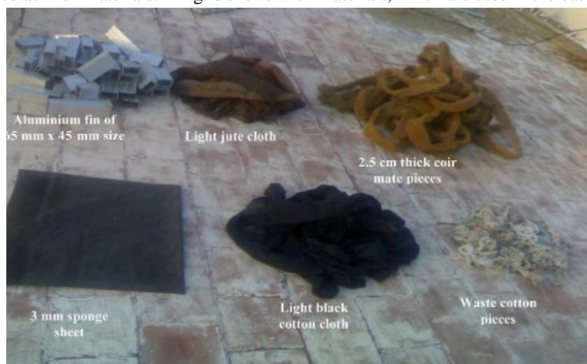
Fig.6. Different type of wick materials were used in the solar still [8]
