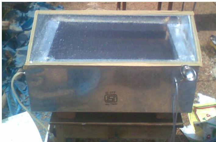
Fig.11. Solar still with PCM [14]
