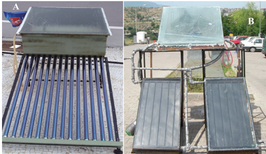
Fig.3. (A) Solar still with evacuated tube collector [4], (B) Solar still with flat plate collector[5].
