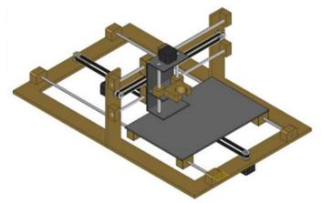
The assembly of chain and motor alignment for X-axis-axis and Z-axis movement. The Motor is used in this mechanism is PMDC, The motor we can operate forward and reverse and so that by changing the direction of rotation as per our requirement we can able to operate the spray gun and its movement.
