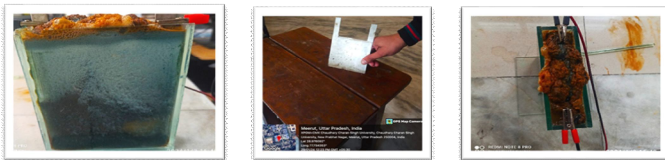
Fig.3 Upper and Side View of Glass Reactor and SS Electrode during Experiments
