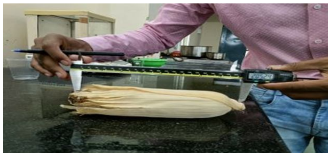
Figure 2. Determination of length of un-dehusked maize cobs using a vernier calliper
