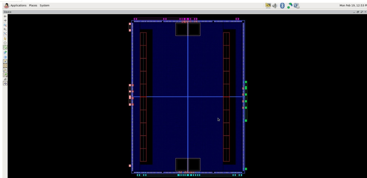
Fig 5. Device planning design of 32 bit LFSR(chip design using Plan Ahead 14.7 )
