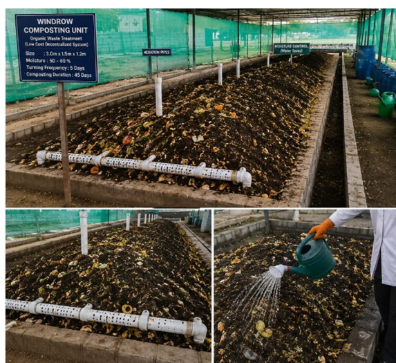
Figure 5. Experimental Windrow Composting Setup
