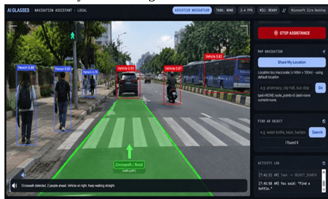
Fig. 7. AI glasses navigation and assistive guidance interface.
