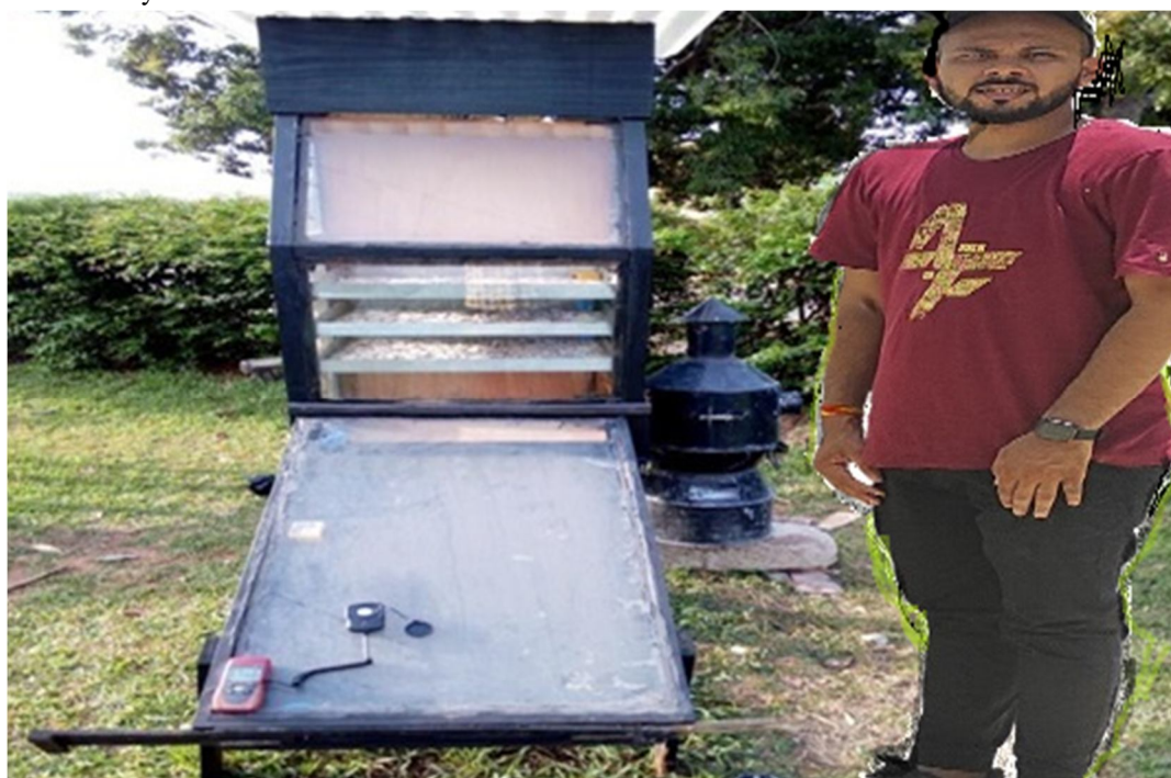
Figure 4: Isometric view of the mixed-mode solar dryer
