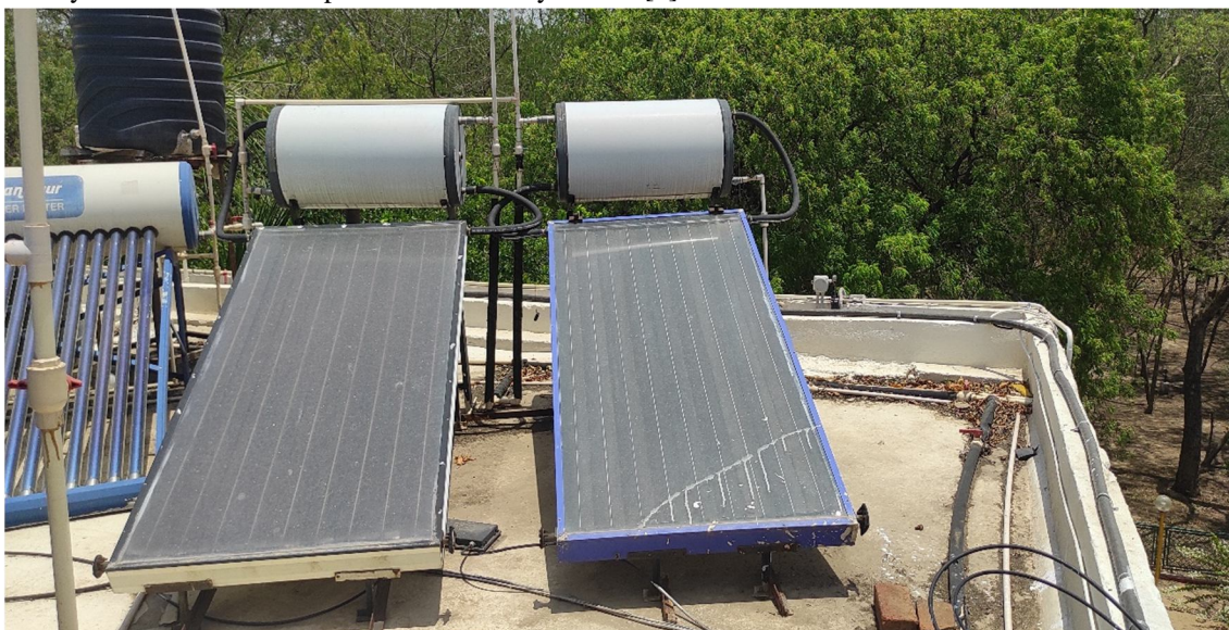
Figure 3: experiments setup water heater with glass cover.
