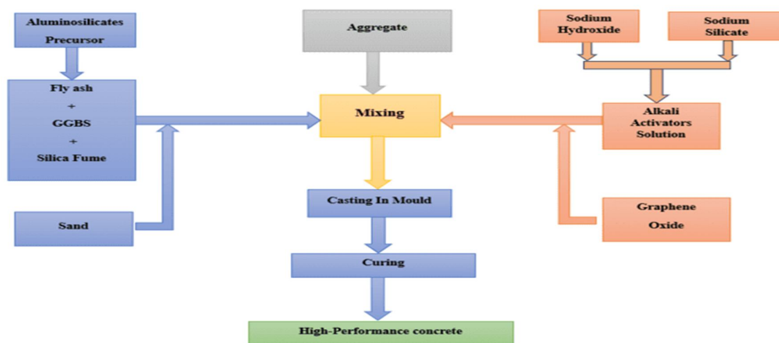
Fig. 1. Flow diagram of the production of Geopolymer concrete
