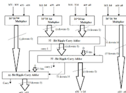
Fig: 32-bit Vedic Multiplier from 16-bit Multiplier
