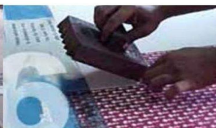
Fig 12: Step 6 – Printing of multi colour.
