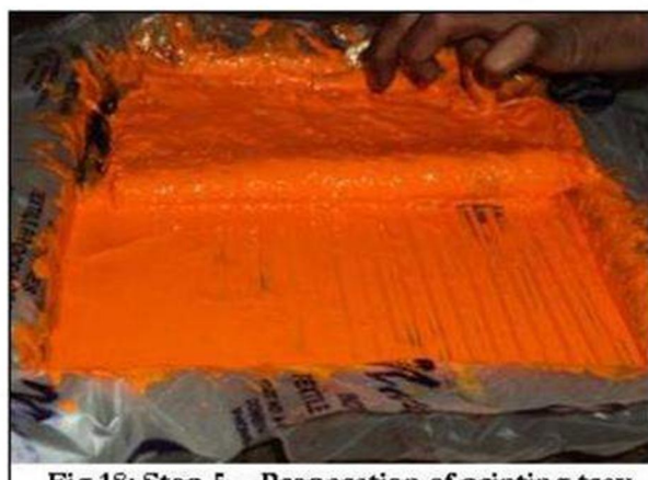
Fig 18: Step 5 – Preparation of printing tray.
