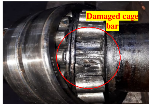
Fig.2 GA drawing of NBM stand 1 Gearbox Fig.3 Failed Bearing of Stand no 1 gearbox.
