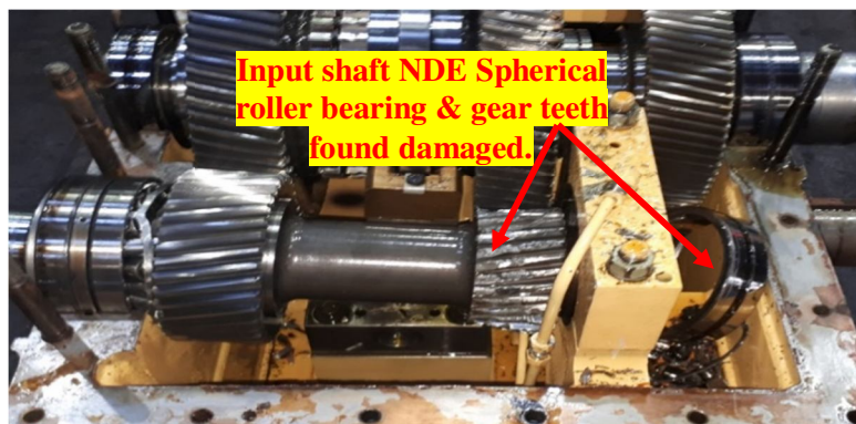
Fig.6 Failed gearbox of stand no 15
