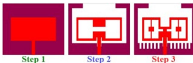
Fig. 2: Different steps of the design and suggested geometry.
