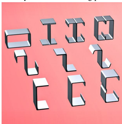
Figure 2 Cold Formed Steel Section[12]
