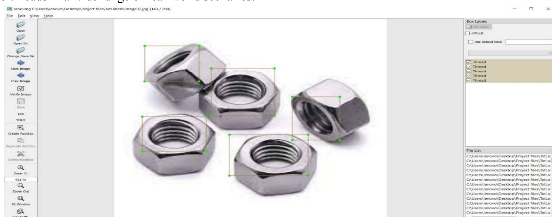
Figure 2: Annotation and Labelling in Labelimg
