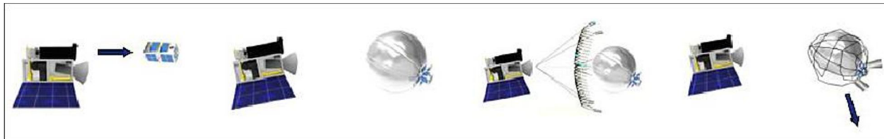
Figure 5: This figure shows the sequence in the net experiment: (a) CubeSat ejection, (b) balloon inflation, (c) net capture, (d) deorbiting (image credit: RemoveDebris consortium) [9]
