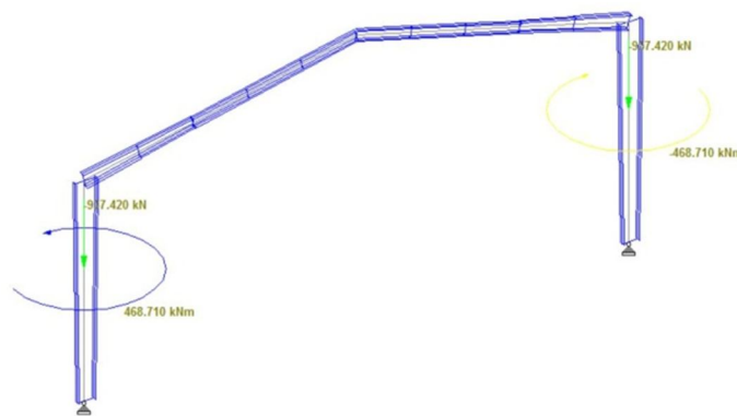
Fig. 11: Factored load and couple moment acting on supporting columns of pre-engineered steel frame
