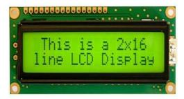
A 16×2 LCD display is a liquid crystal display that can show 16 characters in each of its two rows, providing a total of 32 characters of information. It's commonly used to display alphanumeric information in various electronic devices. A 16x2 LCD is a liquid crystal display module capable of displaying 2 rows with 16 characters each. It is widely used in embedded systems to show textual information such as system status, messages, or sensor outputs.
