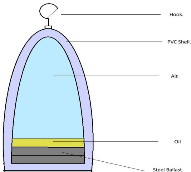
The gravity mass is a single, reusable block designed to operate in both air and water environments. Structurally, the mass consists of a rigid outer shell enclosing ballast material to achieve the required mass, along with a passive buoyancy volume that enables flotation within the water column. The buoyancy configuration is fixed and does not involve active control during operation.
