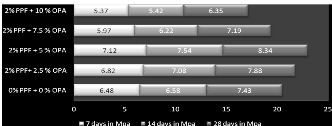
Graph VI Contrast values of flexural strength for 7 days, 14 days & 28 days
