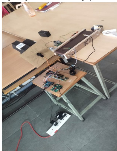
Figure 3: Overview of the prototype of waste segregation and remote garbage level monitoring system
