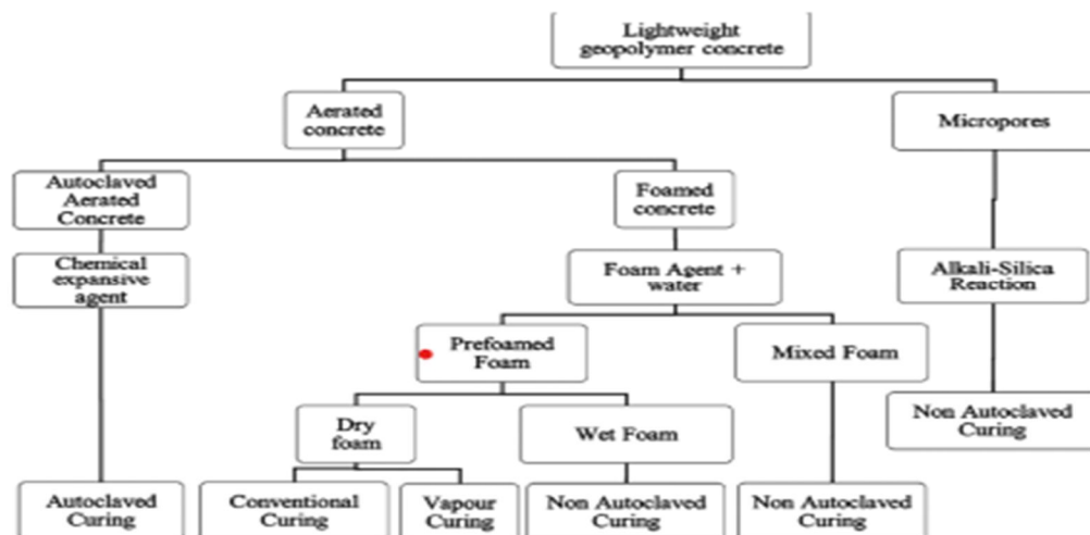
Fig. 2 — Methods to produce lightweight geopolymer concrete.
