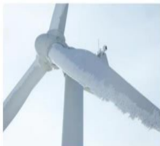
Figure7: Icing on the wind turbine.
