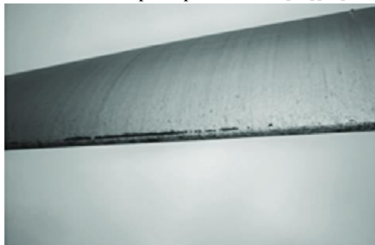
Figure 8: delamination of blade.
