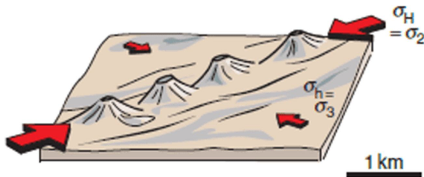
Figure. 9 Stress regime of volcanic vent ( S_v > S_{Hmax} > S_{hmin} )
