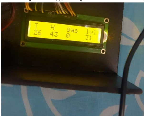
Fig. 6 LCD display shownig various readings
