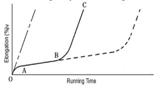
In Figure 2.20, O-A is called "initial wear." At first the wear progresses rapidly, but its ratio is less than 0.1 percent and usually it will cease within 20 hours of continuous operation. A-B is "normal wear." Its progress is slow. B-C is "extreme wear." The limit of <sup>3</sup>allowable wear<sup>2</sup> (the end of its useful life) will be reached during this stage (1.5 to 2.0 percent).
