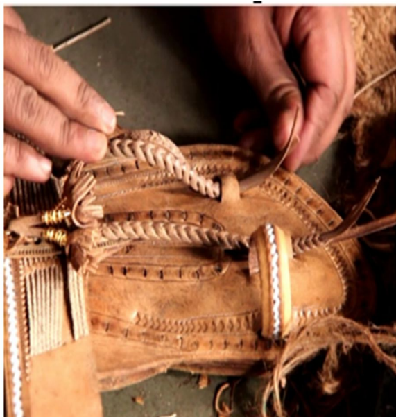
Fig.69 stitching the sole
