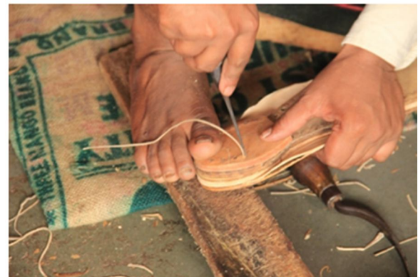
Fig.69 stitching the sole
