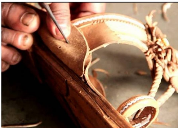
Fig.69 stitching the sole
