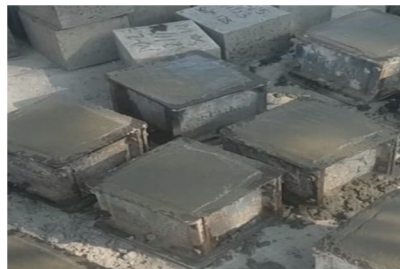
Figure no 4 :Cube Test (150x150x150) mm.
