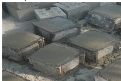
Figure no 4 :Cube Test (150x150x150) mm.
