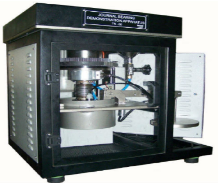
Figure2. 1 Pressure testing equipment (JBTR) [9]
