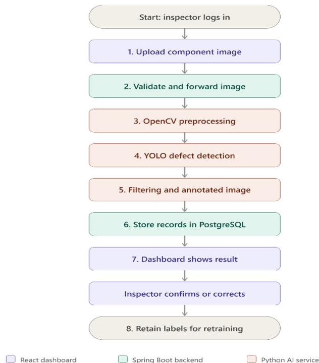
Fig. 2. Flowchart of the inspection workflow.
