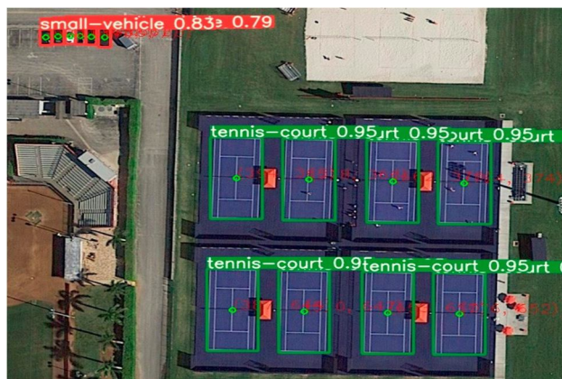
Fig 9. Object detection with YOLOv5[23]
