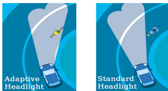
Fig 2: difference between adaptive headlight and standard headlight (cornering lamps)
