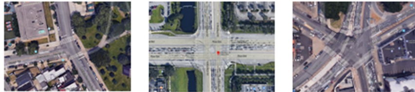
Figure 8: Realistic Data for 3-, 4-, and 6-approach intersections.
