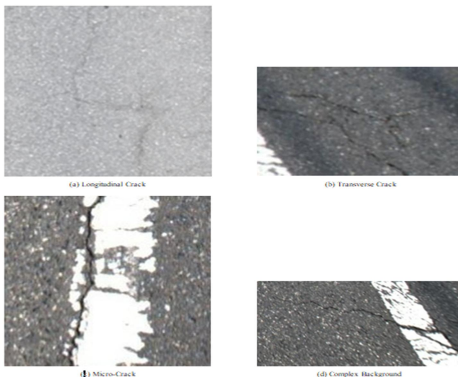
Figure 2: Representative samples from the bridge crack dataset showing different types of cracks and environmental variations
