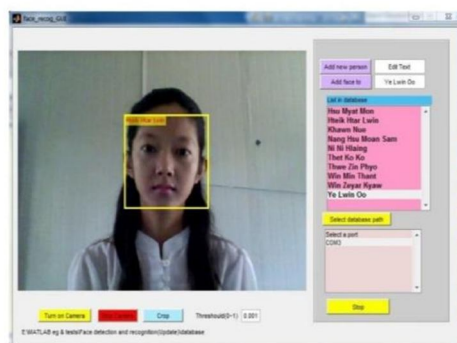
Figure 15. Matlab GUI result when captured face is detected and recognised as authenticated person.
