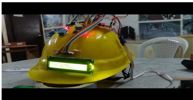
Fig. 4. Hardware Setup os Smart Helmet for Miners
