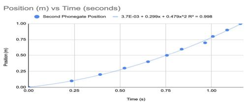
The position vs. time graph depicts the displacement of the cart along the metal ramp over the duration of the experiment. As shown in Figure 1, the graph illustrates how the cart's position changes with time as it descends the ramp. The slope of the graph represents the cart's velocity, with steeper slopes indicating higher velocities. By analyzing the shape of the curve, insights into the cart's acceleration profile can be gleaned, with a steeper curve indicative of greater acceleration.
