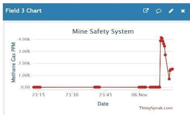
Fig. 10 Methane Gas Data displayed on ThingSpeak
