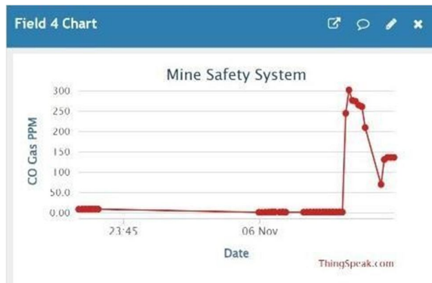
Fig. 11 CO Gas Data displayed on ThingSpeak
