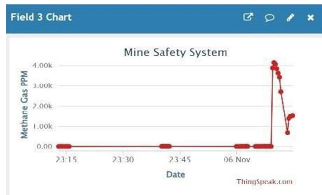
Fig. 10 Methane Gas Data displayed on ThingSpeak
