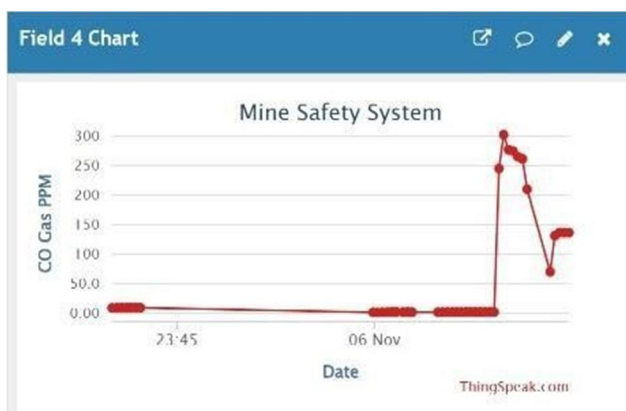
Fig. 11 CO Gas Data displayed on ThingSpeak
