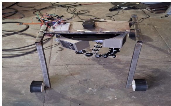
Fig:1.3 Prototype of robotic octopus arm
