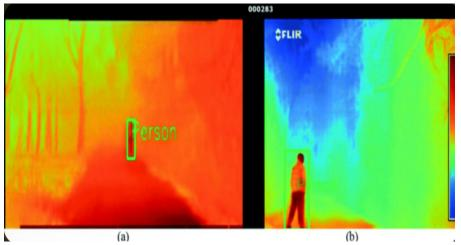
Modern thermal cameras operate in longwave infrared spectrum (8-14 micrometers), corresponding to peak thermal emissions from human body temperature. Advanced systems combine thermal sensors with image processing algorithms to detect human presence at 10-20 meter distances.
