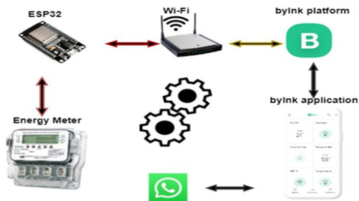
Fig. 3: Mechanism of Smart Energy Monitoring System Using ESP32 Microcontroller [1]
