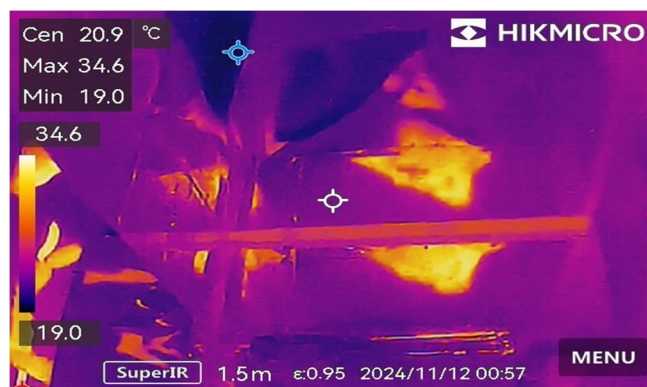
Figure 2 - Thermal Inspection of Ductwork Temperature Variation
