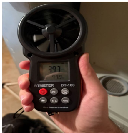
Figure 6 - Intermediate Airflow Test Closer to Ductwork (Test 2)
