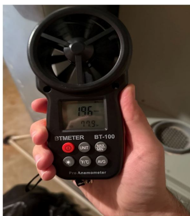
Figure 5 - Initial Airflow Test at Distance from Ductwork (Test 1)
