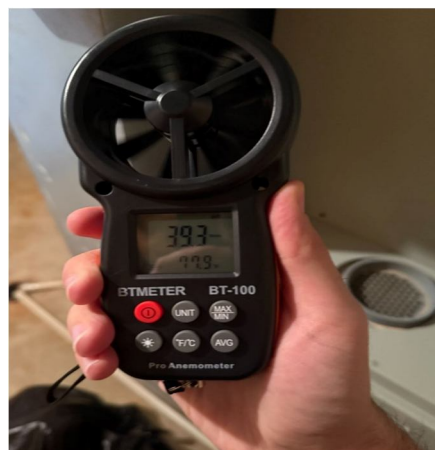
Figure 6 - Intermediate Airflow Test Closer to Ductwork (Test 2)
