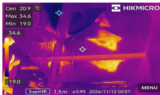
Figure 2 - Thermal Inspection of Ductwork Temperature Variation
