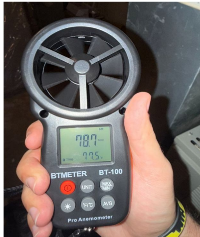
Figure 7 - Increased Airflow Test in Proximity to Ductwork (Test 3)
