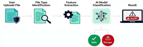
Fig. 4. AegisScan end-to-end file-processing workflow, branching into Safe/Danger verdicts at the classification stage.
