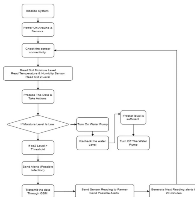
Fig 5.1.1 Working Algorithm Of Trinetra
