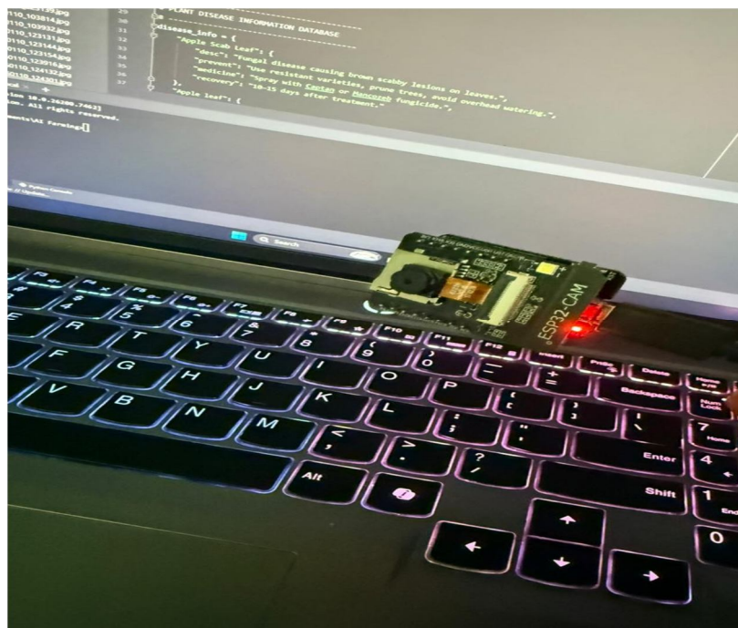
Figure 7:ESP32 CAM Module Integrated with Real-Time Plant Disease Detection System
