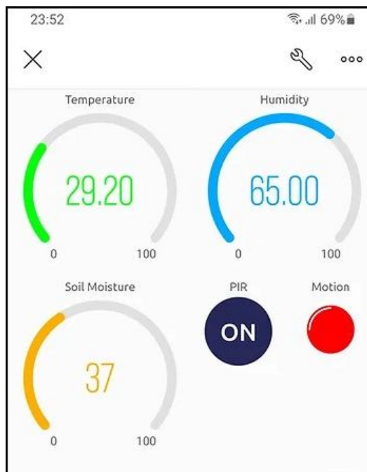
Fig. 1 Blynk interface showing reading of sensors
